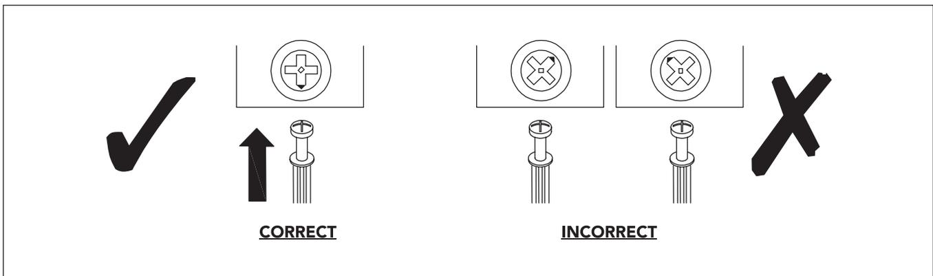
Quickfit head should be in the centre of the cam lock when the two panels are joined. Cam lock should be inserted before quickfit.
