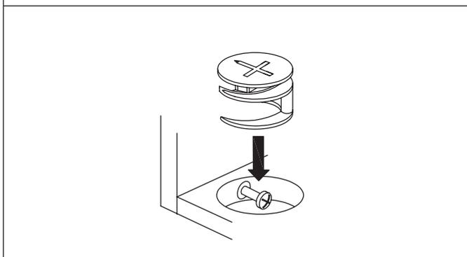
Turn cam lock clockwise to tighten.
