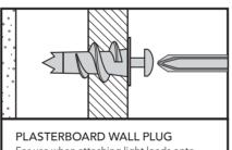
For use when attaching light loads onto plasterboard partitions
