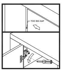
Turn the screw counterclockwise a little as shown to make the gap small.
