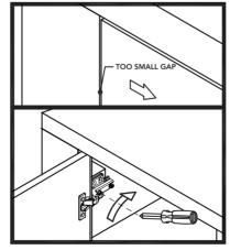
Turn the screw clockwise a little as shown to make the gap big.
