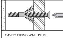
For use with plasterboard partitions or hollow wooden doors.
