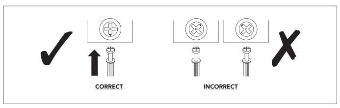
Quickfit head should be in the centre of the cam lock when the two panels are joined. Cam lock should be inserted before quickfit.
