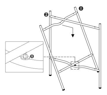
**STEP 2:** Use the Allen Key (C) to secure a Screw (A) through the bar intersection with a Washer (B) placed between the bars.
