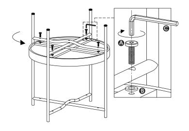
**STEP 5:** Place the second Tray (3) under the Legs and use the Allen Key (C) to secure a Screw (A) through the bar intersection with a Washer (B) placed between the bars. Repeat 4 times.
