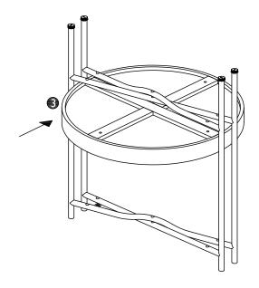
**STEP 4:** Twist the legs back to a right angle. Use the Allen Key (C) to secure a Screw (A) through the bar intersection with a Washer (B) placed between the bars. Repeat 4 times.
