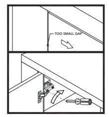
Turn the screw clockwise a little as shown to make the gap big.
