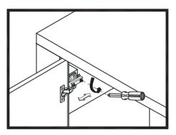
Loosen the screw indicated a little, adjust the hinge to right position (see Step 2A & 2B), then tighten screw.
