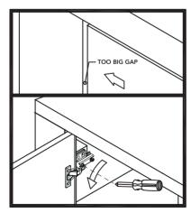
Turn the screw counterclockwise a little as shown to make the gap small.
