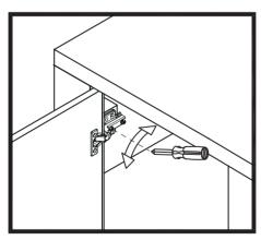
Loosen or tighten the screw indicated a little to adjust the gap between door and leg (see Step 3A & 3B).
