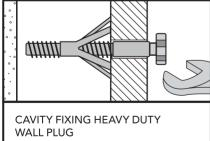
For use when fitting or supporting heavy loads such as shelving and wall cabinets.
