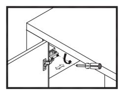
Loosen the screw indicated a little, adjust the hinge to right position (see Step 2A & 2B), then tighten screw.
