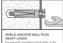
use with heavier loads such as TV & HiFi speakers and satellite dishes, etc.
