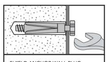
SHIELD ANCHOR WALL PLUG HEAVY LOADS For use with concrete or brick walls, or for use with heavier loads such as TV & HiFi speakers and satellite dishes, etc.
